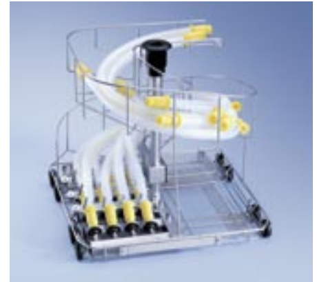
E 461/2 Mobile unit For use in G 7892, G 7882 CD, PG 8535, PG 8536 • For 12 breathing tubes up to 1.5 m long, fitted on a spiral rack • 1 x E 432 holder for • 4 breathing tubes each • 3 x E 433 holders for 4 silicone tubes, enclosed • 1 x E 434 holder for 4 paediatric breathing tubes • 1 x E 430/1 mesh tray • 1 x A 3 cover net • Connection for hot-air drying unit • Holder for ML/2 magnetic strip for automatic mobile unit recognition • H 502, W 535, D 515 mm
