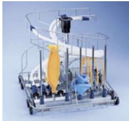
E 436/3 Mobile unit For use in PG 8536 • For approx. 3 AN sets • 8 spring nozzles for breathing tubes with max. length of 1.5 m • Fitted on a spiral rack • Connection for hot-air drying unit • Holder for ML/2 magnetic strip for automatic mobile unit recognition • H 507, W 535, D 515 mm
